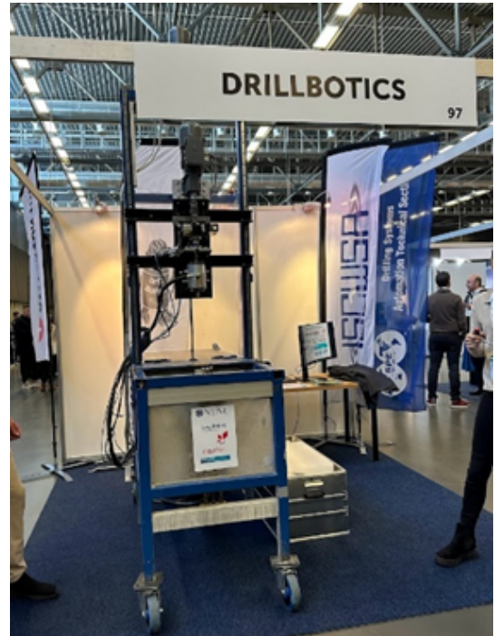
Model Drilling rig by the Stavanger student Chapter who won the Drillbotics 2021 competition
