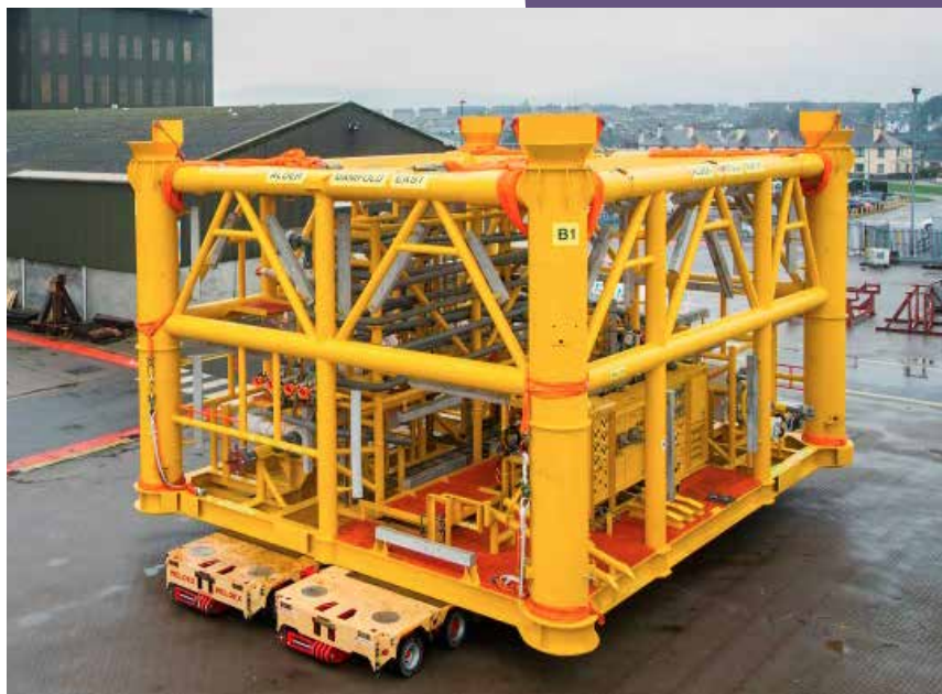
The Alder subsea manifold leaving its U.K. fabrication yard earlier this year. It houses a unique subsea cooling loop to reduce the temperature of production fluids before they enter the pipeline and a subsea High Integrity Pressure Protection System that manages the pressure between the reservoir and the receiving facilities.
