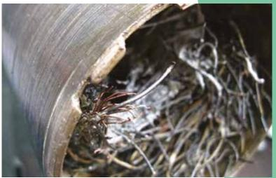
Monoconductor cable recovered inside mill bit.
