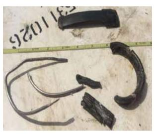
Small lengths of slickline and parts of an Universal Pulling Tool recovered inside AFH plug.
