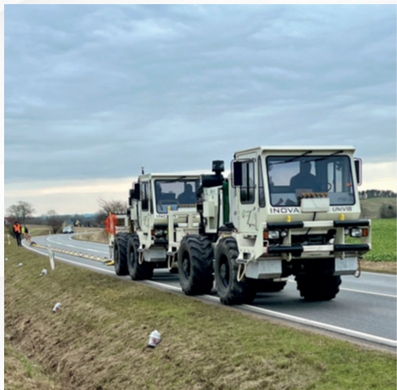
Figure 2. Two vibrators were used for the seismic campaign. The seismic data was acquired along all accessible roads in the area.
