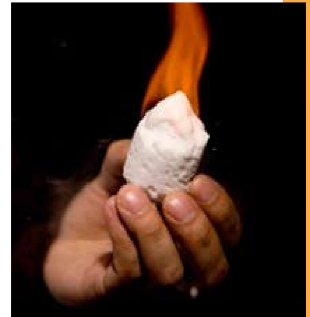
The so-called "burning snowball" – methane gas and water in the form of a hydrate is combustible
