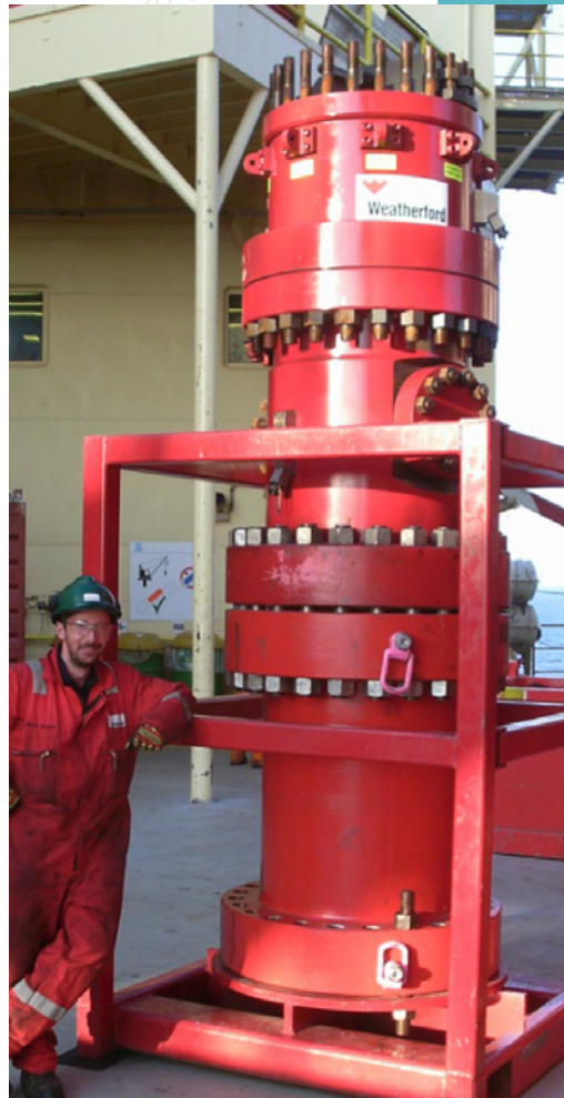
A RCD spool is a part of the MPD equipment which makes it possible to add backpressure on the wellbore during drilling operations.
