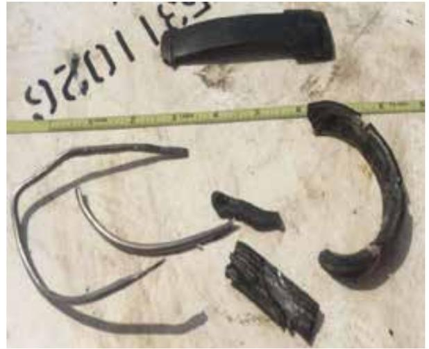
*Small lengths of slickline and parts of an Universal Pulling Tool recovered inside AFH plug.*
