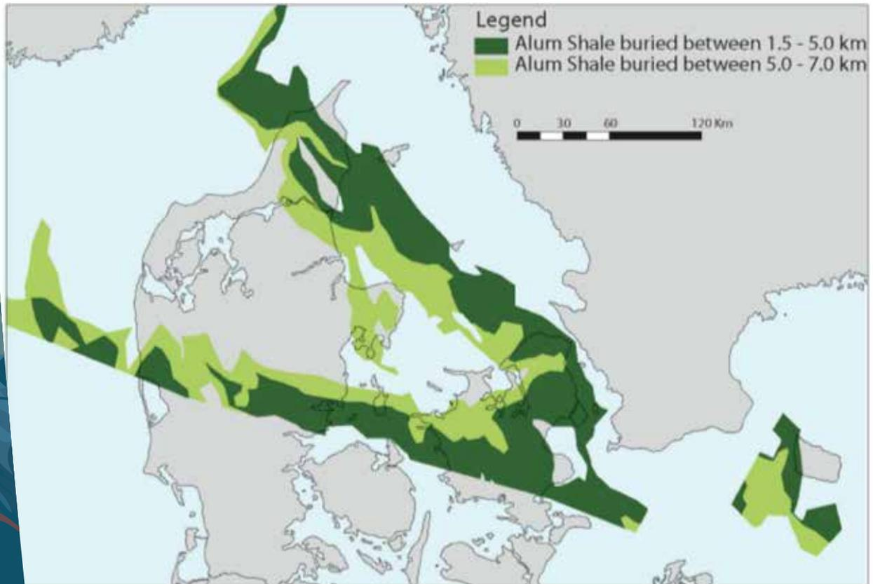
European shale gas exploration is still in its early phase. In many countries the oil and gas industry has focused on thick organic rich Palaeozoic shales known as important source rocks for conventional oil and gas fields. In Denmark shale gas research and exploration is also focused on the Lower Palaeozoic shales and two licences have been awarded to Total E&P. The first exploration well for shale gas is scheduled to be drilled in northern Jutland mid-2014.
